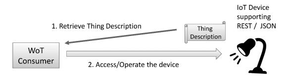
In the figure above, a smart lamp supporting REST / JSON is described by a TD. Once a WoT Consumer obtained a TD for the lamp and understand the TD, the WoT Consumer is ready to interact with the lamp and be able to turn on/off, set brightness, activate embedded motion sensor, etc.
